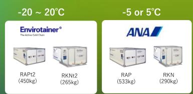
\*The inside temperature of container will be maintained  $\pm 3^{\circ}$ C when the ambient temperature is more than 5°C and less than 25°C higher than the container set temperature. If the difference between the container set temperature and the outside temperature is larger than the said range, the temperature may deviate from the desired range.
